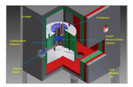
5 L uranyl sulfate solution in a 304SS vessel
